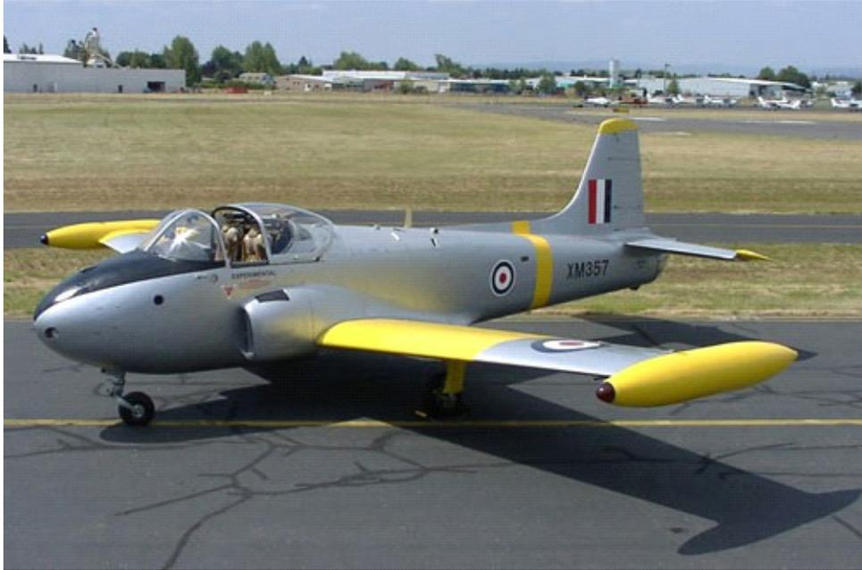
In June 1957, an order was duly placed for the first 40 of the developed **Jet Provost T3**, featuring a more powerful Armstrong Siddeley Viper jet engine, ejector seats, a redesign of the airframe, and a shortened and strengthened version of the retractable tricycle undercarriage. In total, 201 T3s were delivered between 1958 and 1962.
